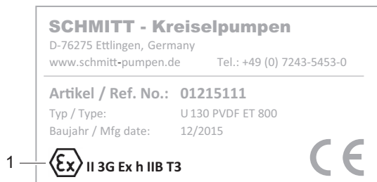
Fig. 2 ATEX type plate (example)
