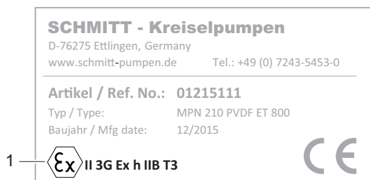
Fig. 2 ATEX type plate (example)
